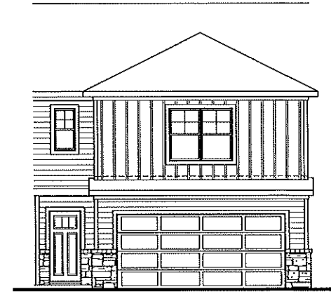
Front Elevation 'A-1' At Interior Unit Condition SCALE: 1/4"=1'-0" AT 22'00" LAYOUT 1/8"=1'-0" AT 10'00" LAYOUT
