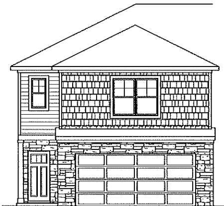
Front Elevation 'A-4' At End Unit Condition - L SCALE: 1/4"=1'-0" AT 22'X34' LAYOUT 1/8"=1'-0" AT 15'X17' LAYOUT
