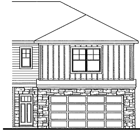
Front Elevation 'A-3' At End Unit Condition - R SCALE: 1/4"=1'-0" AT 22'X34' LAYOUT 1/8"=1'-0" AT 15'X17' LAYOUT
